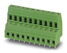
Printed circuit terminal block, nominal current: 8 A, rated voltage: 160 V, pitch: 3.81 mm, no. of positions: 10, mounting: Soldering, type of connection: Screw connection, connection direction from the conductor to the PCB:  $0^{\circ}$
