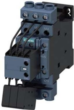
capacitor contactor, AC-6b 33 kVAr, / 400 V, 3-pole, 200-280 V AC/DC, 50/60 Hz, with integrated varistor, auxiliary contacts: 1 NO + 2 NC, screw terminal, size: S0
