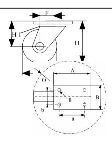
Castor Assembly: Pressed stainless steel -AISI 304-. Swivel on two rows of balls.
