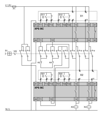
When operator 1 is absent: replace terminal block X1 by X3 and physically remove the two-hand control station.
