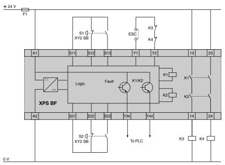
ESC: External start conditions. Y1-Y2: feedback loop
