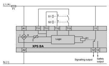
S1 and S2: pushbuttons. Must not be used for applications (presses) which require a type III C module (XPS BC).
