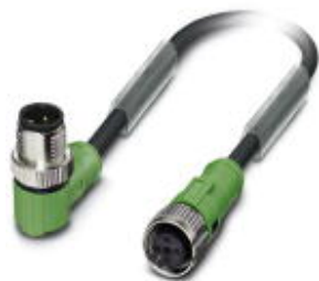
Sensor/Actuator cable, 3-position, PUR halogen-free, black-gray RAL 7021, Plug angled M12 SPEEDCON, A-coded, on Socket straight M12 SPEEDCON, A-coded, Cable length: 0.6 m
