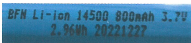
电池组铭牌 View of the battery nameplate
