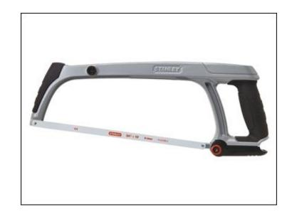
The Stanley FatMax hacksaw with a durable die-cast aluminium body that is both lightweight and strong. It has a thumb grip for a more accurate cut, and a bi-material soft grip for comfort. The saw has an adjustable thumb dial tension mechanism inside its handle, and this spring loaded tension device gives up to 150kg blade tension for ease of use.
