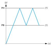
Pressure Time Adjustable value High point Below point (y) (x) (1) PH: PB:
