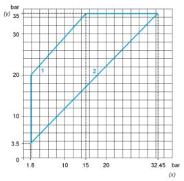
Rising pressure Falling pressure Maximum differential (y) (x) 1: 2: Minimum differential
