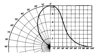
Figure 8: Relative Luminous Intensity vs. Angular Displacement, HLMP-K101
