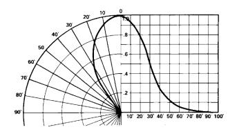
Figure 10: Relative Luminous Intensity vs. Angular Displacement, HLMP-K105
