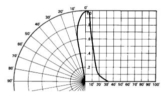
Figure 9: Relative Luminous Intensity vs. Angular
