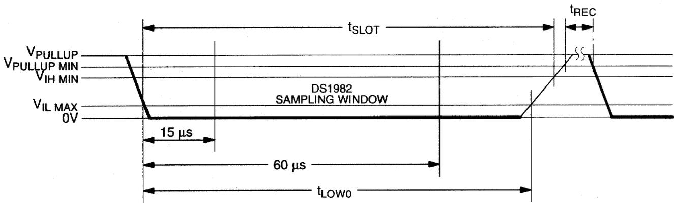
$$60 \mu s \leq t_{LOW0} < t_{SLOT} < 120 \mu s$$
