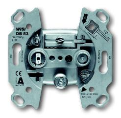
Broadband technology 47-2.150 MHz. SAT connection designed as screwable F-male plug. with remote feed via F-bush For DVB-T and broadband-cable-systems. For analogue and digital transmission. With claw.
