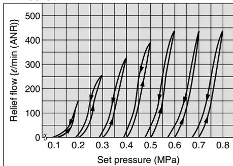
Note) The graph above shows the relief flow when the set pressure rises and falls from 0.1 MPa.
