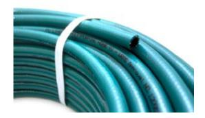
RS Pro multi-purpose PU lined hose delivers exceptional durability and flexibility. Manufactured in the UK, this anti-abrasive Polyurethane (PU) and PVC compound hose is reinforced with polyester yarn. RS Pro multi-purpose hose is ideal for pneumatic tools in general, abrasive applications and water-based paint sprayers. The PU lining material also has WRAS approval for use with drinking water application.
