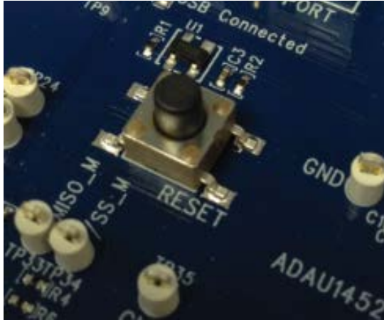
Figure 68. Manual Reset Push-Button and Reset Generator IC
