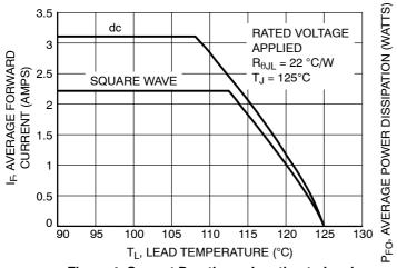
Figure 4. Current Derating - Junction to Lead
