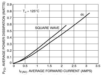
Figure 5. Forward Power Dissipation
