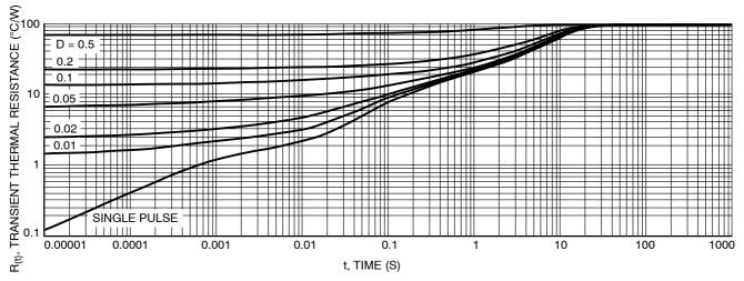
Figure 7. Thermal Response, Junction to Ambient (min pad)
