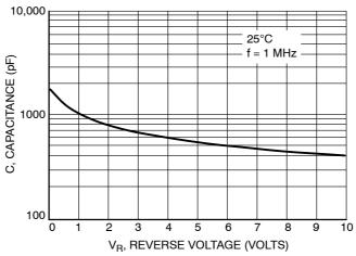
Figure 6. Typical Capacitance
