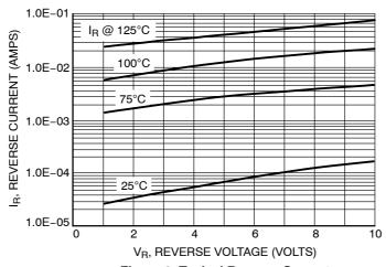
Figure 3. Typical Reverse Current
