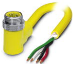
Sensor/Actuator cable, 4-position, PVC, Yellow RAL 1021, Plug angled 7/8"-16UNF, A-coded, on free cable end, Cable length: 6 m
