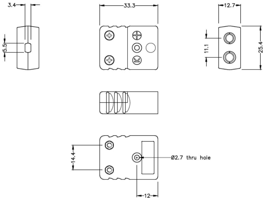
**Standard Hi-Temp Plastic in-line Socket - HTP**
