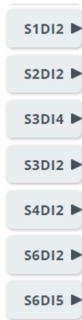
Figure 27: Digital input blocks – e. g.: port 3 provides two digital inputs: one on pin 2 and another one on pin 4
