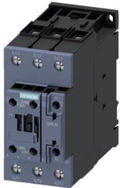
power contactor, AC-3e/AC-3, 41 A, 18.5 kW / 400 V, 3-pole, 20-33 V AC/DC, 50/60 Hz, with integrated varistor, auxiliary contacts: 1 NO + 1 NC, screw terminal, size: S2, upright mounting position
