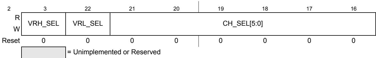
Figure 10-19. ADC Command Register 1 (ADCCMD_1)
