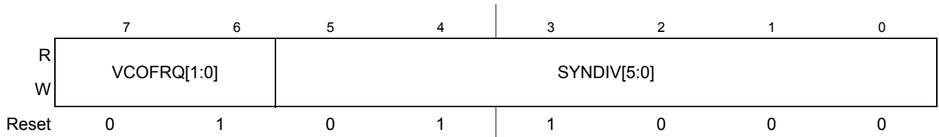
Figure 7-5. S12CPMU_UHV_V6 Synthesizer Register (CPMUSYNR)
