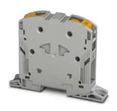
Feed-through terminal block, Connection method: Push-in connection, Cross section: 25 mm² - 95 mm², AWG: 4 - 3/0, Width: 25 mm, Height: 99.8 mm, Color: gray, Mounting type: Direct screw connection
