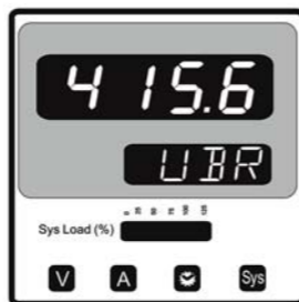
Screen 6 : Line to Line Voltage (Voltage between B and R phase)
