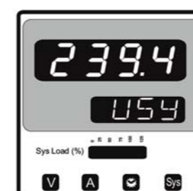
Screen 14 : System Voltage
