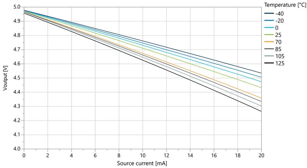
Figure 33-24. I/O Pin Output Voltage vs. Source Current ( $T=25^{\circ}C$ )
