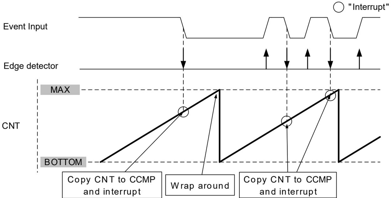
It is recommended to write zero to the TCBn.CNT register when entering this mode from any other mode.
