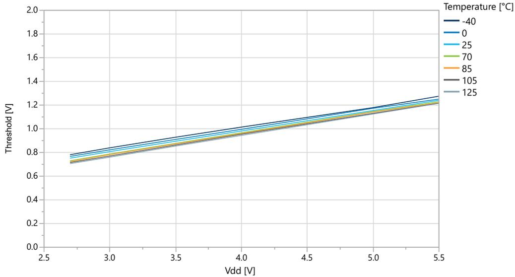
**Figure 33-16. I/O Pin Input Threshold Voltage vs.  $V_{DD}$  ( $T=25^{\circ}\text{C}$ )**
