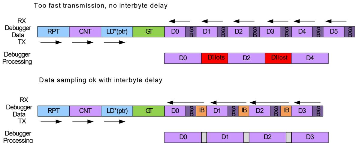
In [Figure 31-18](#), GT denotes the Guard Time insertion, SB are Stop bits and IB is the inserted interbyte delay. The rest of the frames are data and instructions.
