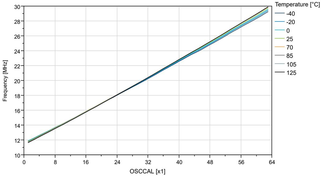
Figure 33-54. OSC20M Internal Oscillator: Frequency vs. Temperature
