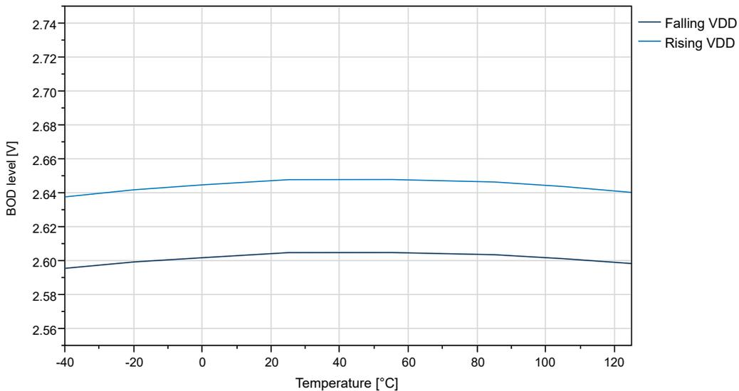
**Figure 33-35. BOD Threshold vs. Temperature (Level 4.3V)**
