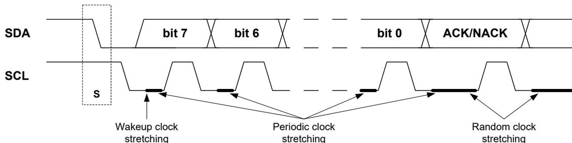
**Note:** Clock stretching is not supported by all I<sup>2</sup>C slaves and masters.
