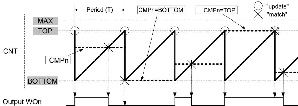
The TCA<sub>n</sub>.PER register defines the PWM resolution. The minimum resolution is 2 bits (TCA.PER=0x0003), and the maximum resolution is 16 bits (TCA.PER=MAX).
