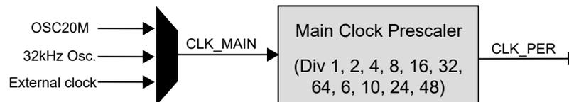
The Main Clock and Prescaler configuration registers (CLKCTRL.MCLKCTRLA, CLKCTRL.MCLKCTRLB) are protected by the Configuration Change Protection Mechanism, employing a timed write procedure for changing these registers.
