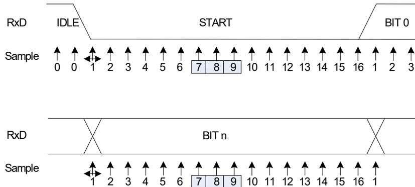
The transmission baud rate must be set up in relation to the selected UPDI clock, which can be adjusted by UPDICKSEL in UPDI.ASI\_CTRLA. See [Table 31-2](#) for recommended maximum and minimum baud rate settings.
