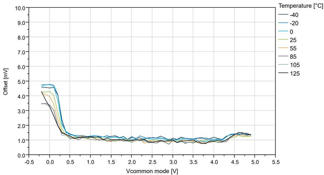
**Figure 33-49. Offset vs.  $V_{CM}$  - 10 mV to 50 mV ( $V_{DD}=5V$ ,  $T=25^{\circ}C$ )**
