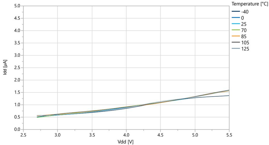
**Figure 33-33. BOD Current vs. V<sub>DD</sub> (Sampled BOD at 1 kHz)**
