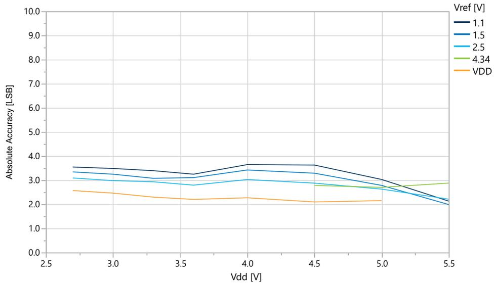
**Figure 33-37. Absolute Accuracy vs.  $V_{ref}$  ( $V_{DD}=5.0V$ ,  $f_{ADC}=115$  kps), REFSEL = Internal Reference**
