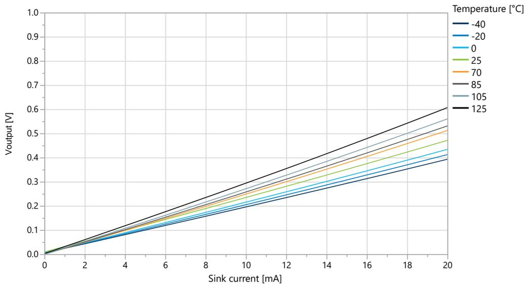
**Figure 33-21. I/O Pin Output Voltage vs. Sink Current (T=25°C)**
