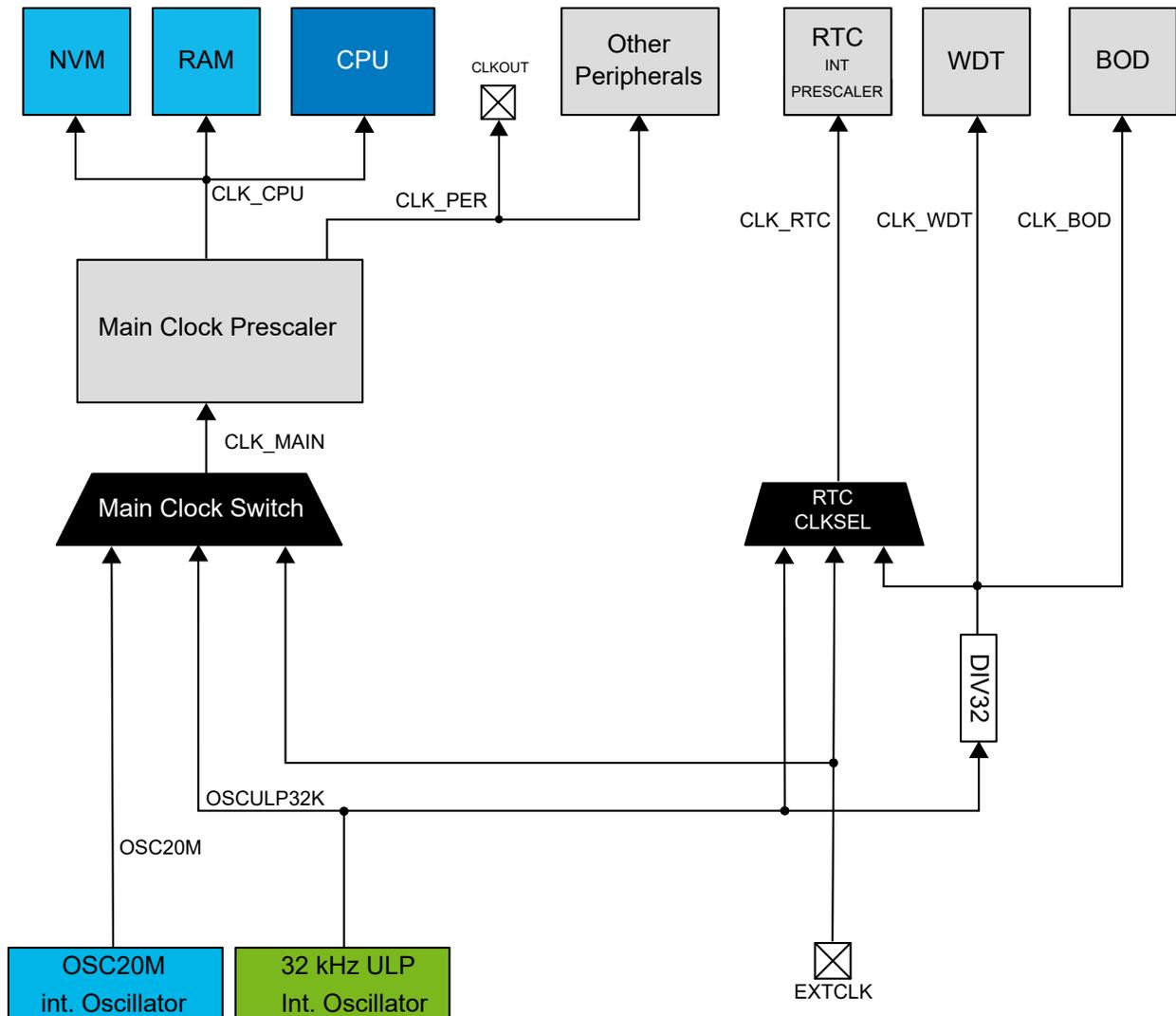
The clock system consists of the Main Clock and other asynchronous clocks:
