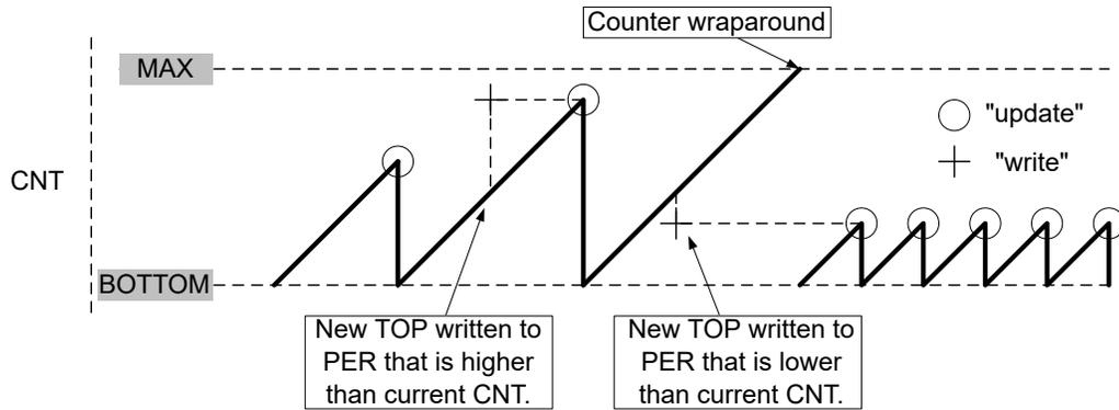
A counter wrap-around can occur in any mode of operation when up-counting without buffering. This is due to the fact that the registers TCA<sub>n</sub>.CNT and TCA<sub>n</sub>.PER are continuously compared: if a new TOP value is written to TCA<sub>n</sub>.PER that is lower than current TCA<sub>n</sub>.CNT, the counter will wrap first, before a compare match happens.
