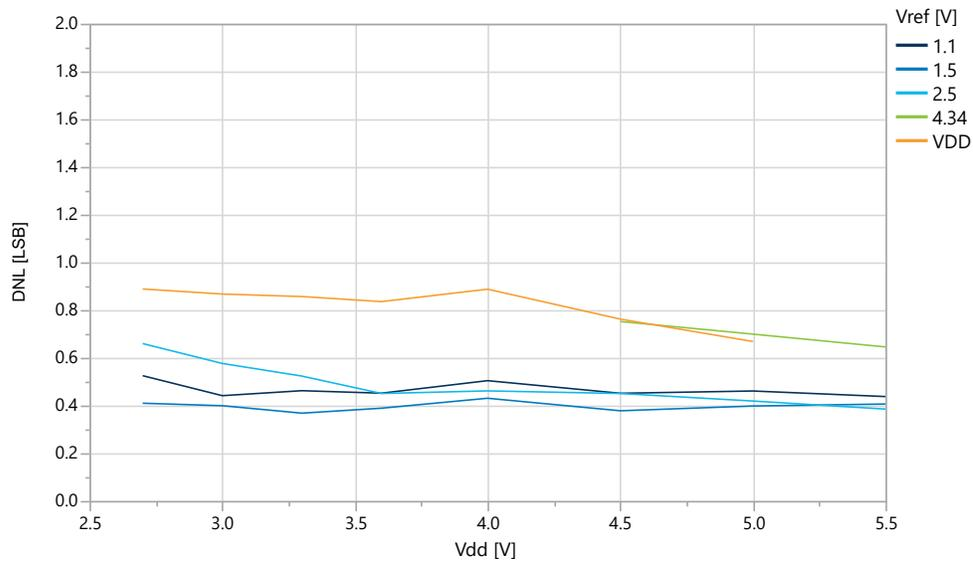
**Figure 33-39. DNL vs.  $V_{ref}$  ( $V_{DD}=5.0V$ ,  $f_{ADC}=115$  kps), REFSEL = Internal Reference**
