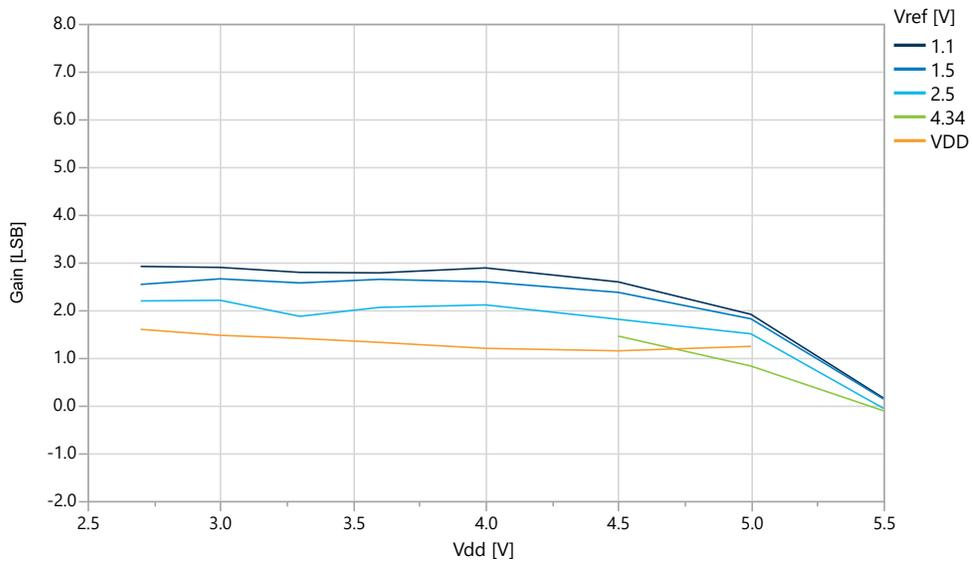
**Figure 33-41. Gain Error vs.  $V_{ref}$  ( $V_{DD}=5.0V$ ,  $f_{ADC}=115$  ksp/s), REFSEL = Internal Reference**
