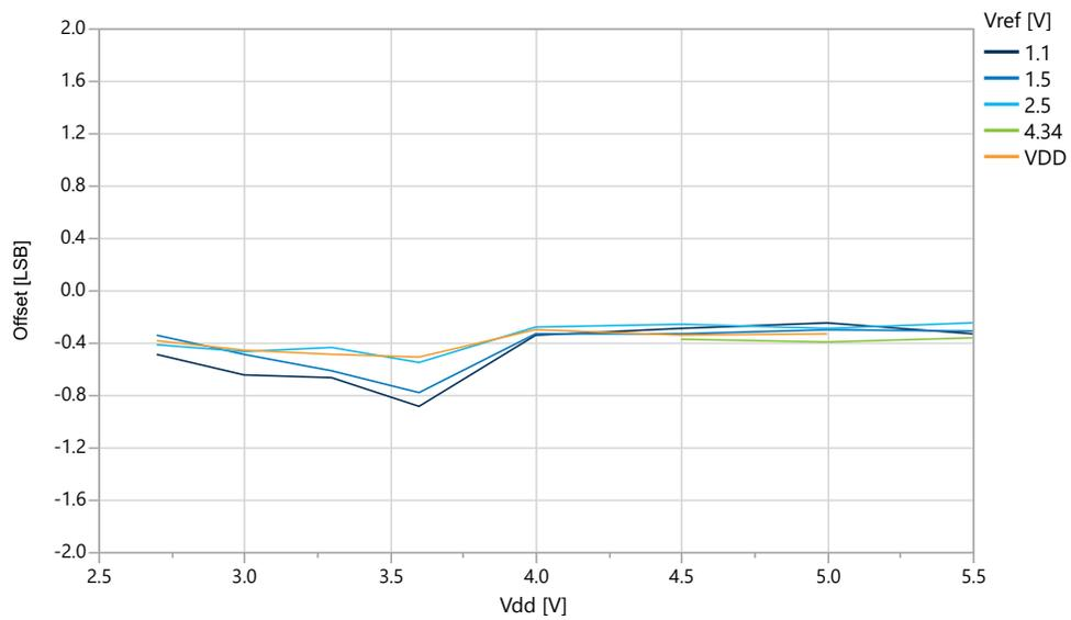
**Figure 33-45. Offset Error vs.  $V_{ref}$  ( $V_{DD}=5.0V$ ,  $f_{ADC}=115$  kpsps), REFSEL = Internal Reference**
