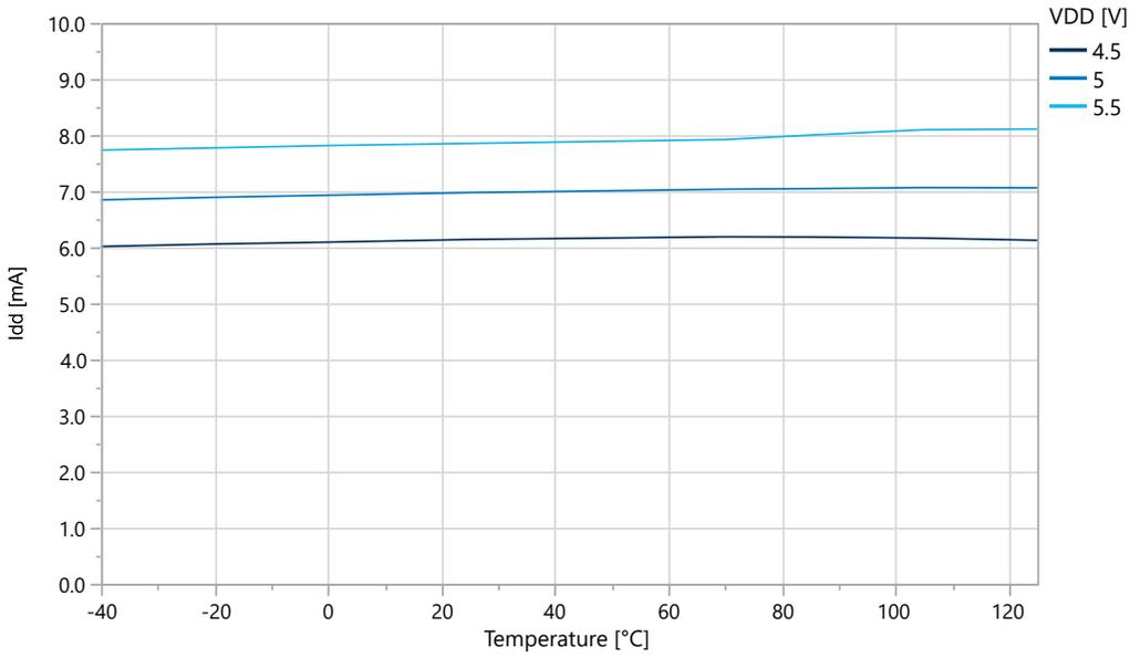
Figure 33-4. Active Supply Current vs. V<sub>DD</sub> (f=[1, 16] MHz OSC20M) at T=25°C
