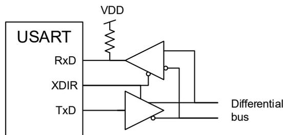
The XDIR pin goes high one baud clock cycle in advance of data being shifted out, to allow some guard time to enable the external line driver. The XDIR pin will remain high for the complete frame including Stop bit(s).
