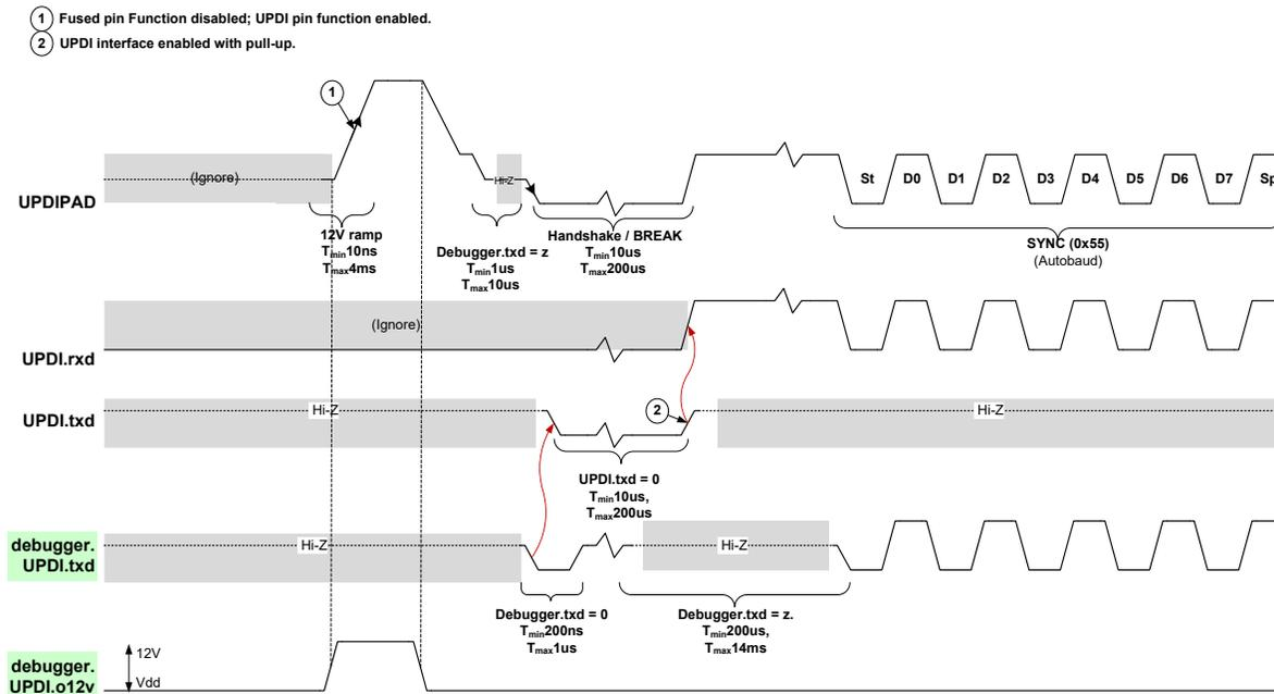
When enabled by 12V, only a POR will disable the UPDI configuration on the  $\overline{\text{RESET}}$  pin, and restore the default setting. If issuing a UPDI Disable command through the UPDIDIS bit in UPDI.CTRLB, the UPDI will be reset and the clock request will be canceled, but the  $\overline{\text{RESET}}$  pin will remain in UPDI configuration.
