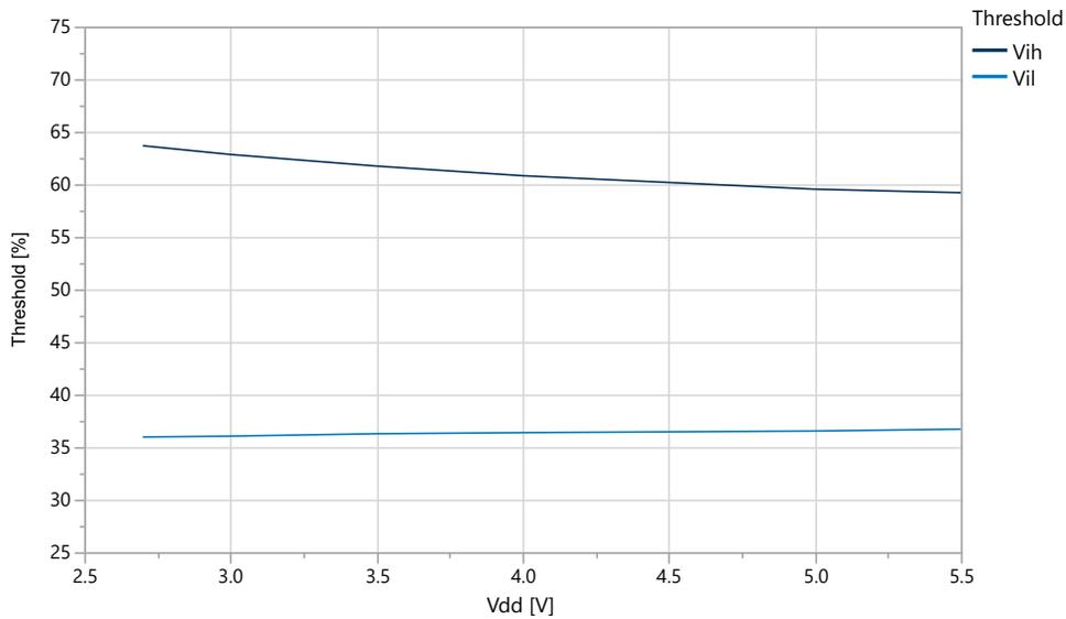
Figure 33-17. I/O Pin Input Threshold Voltage vs.  $V_{DD}$  ( $V_{IH}$ )
