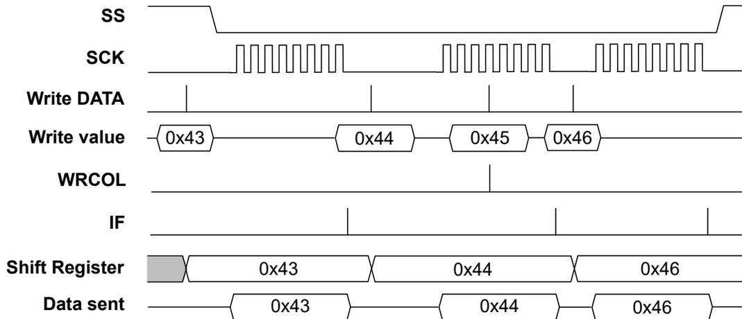
The figure shows three transfers and one write to the DATA register while the SPI is busy with a transfer. This write will be ignored and the Write Collision Flag (WRCOL in SPIn.INTFLAGS) is set.
