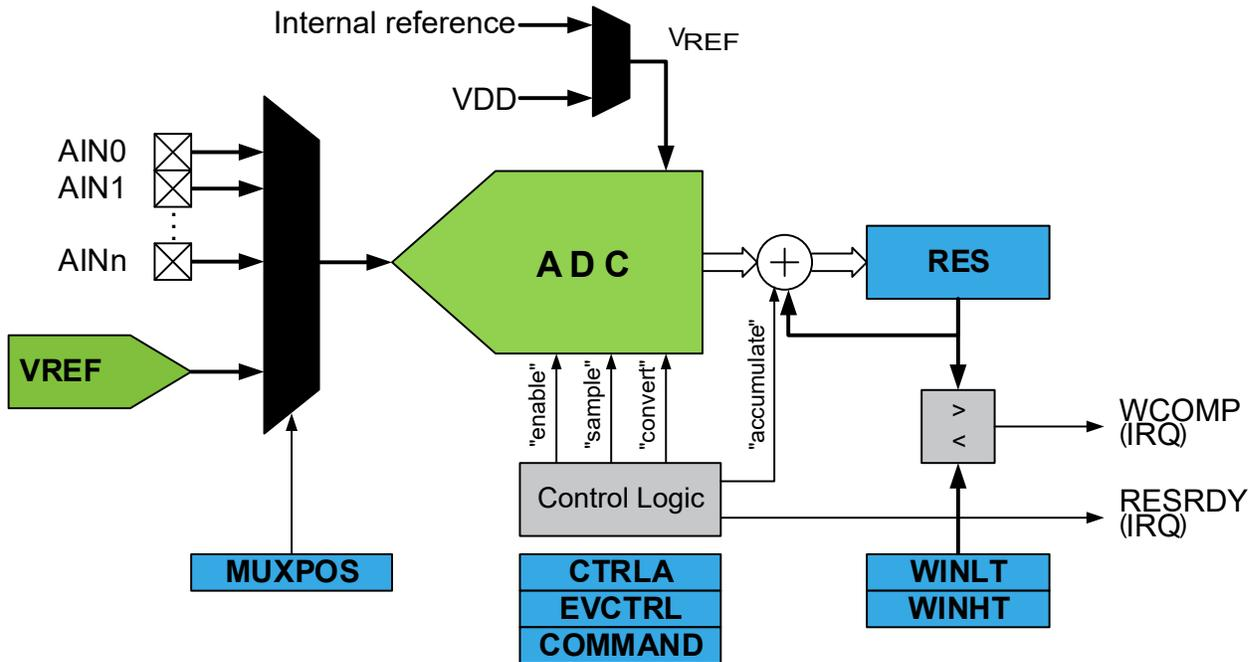
The analog input channel is selected by writing to the MUXPOS bits in the MUXPOS register (ADC.MUXPOS). Any of the ADC input pins, GND, can be selected as single-ended input to the ADC. The ADC is enabled by writing a '1' to the ADC ENABLE bit in the Control A register (ADC.CTRLA). Voltage reference and input channel selections will not go into effect before the ADC is enabled. The ADC does not consume power when the ENABLE bit in ADC.CTRLA is '0'.
