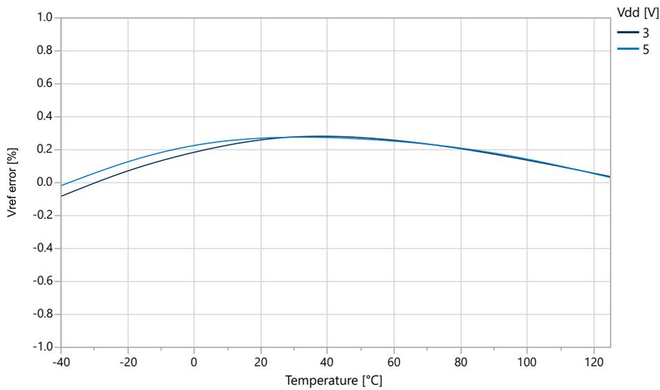
Figure 33-29. Internal 2.5V Reference vs. Temperature
