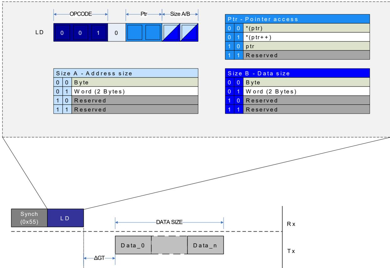
The figure above shows an example of a typical LD sequence, where data is received after the Guard Time period. Loading data from the UPDI Pointer register follows the same transmission protocol.
