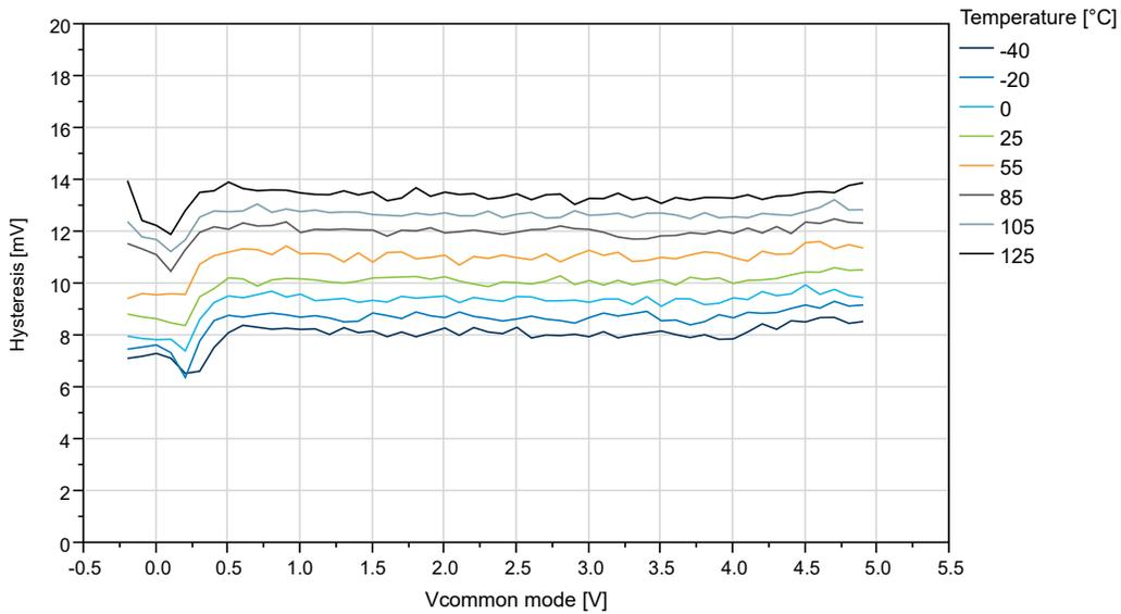
Figure 33-47. Hysteresis vs.  $V_{CM}$  - 10 mV to 50 mV ( $V_{DD}=5V$ ,  $T=25^{\circ}C$ )
