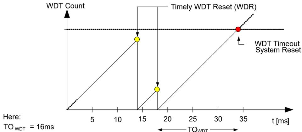
Normal mode is enabled as long as the WINDOW bit field in the Control A register (WDT.CTRLA) is 0x0.
