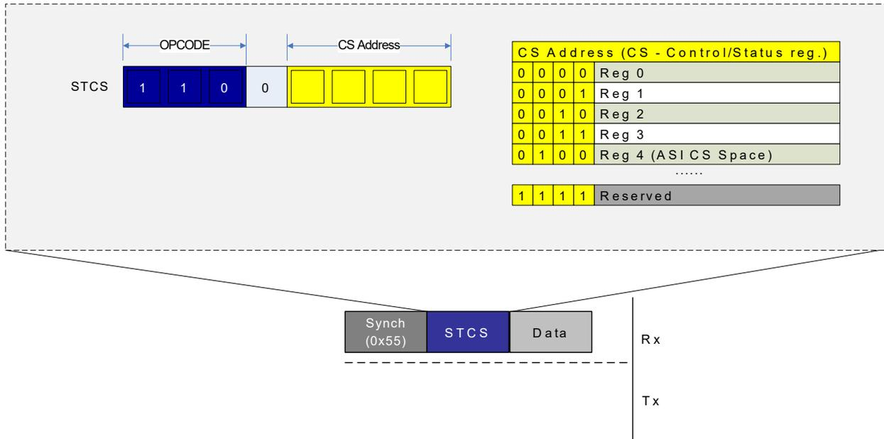
Figure 31-14 shows the data frame transmitted after the SYNCH and instruction frames. There is no response generated from the STCS instruction, as is the case for ST and STS.
