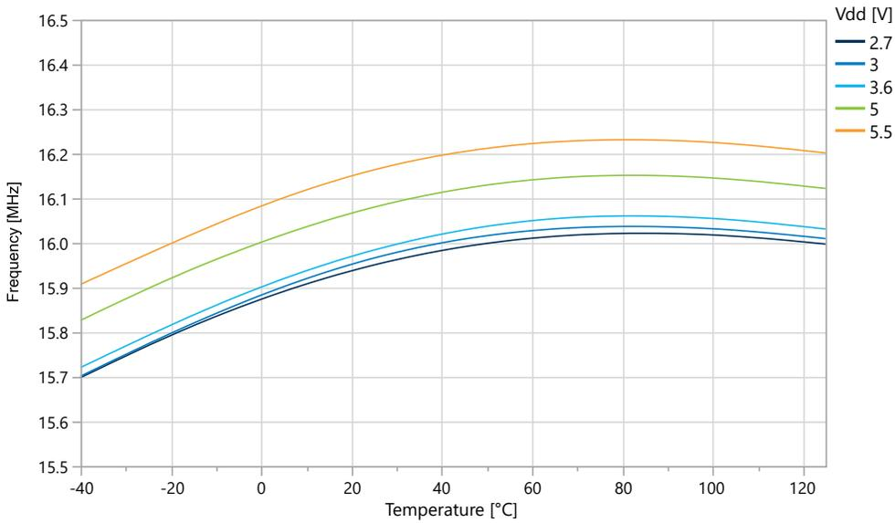
**Figure 33-55. OSC20M Internal Oscillator: Frequency vs. V<sub>DD</sub>**
