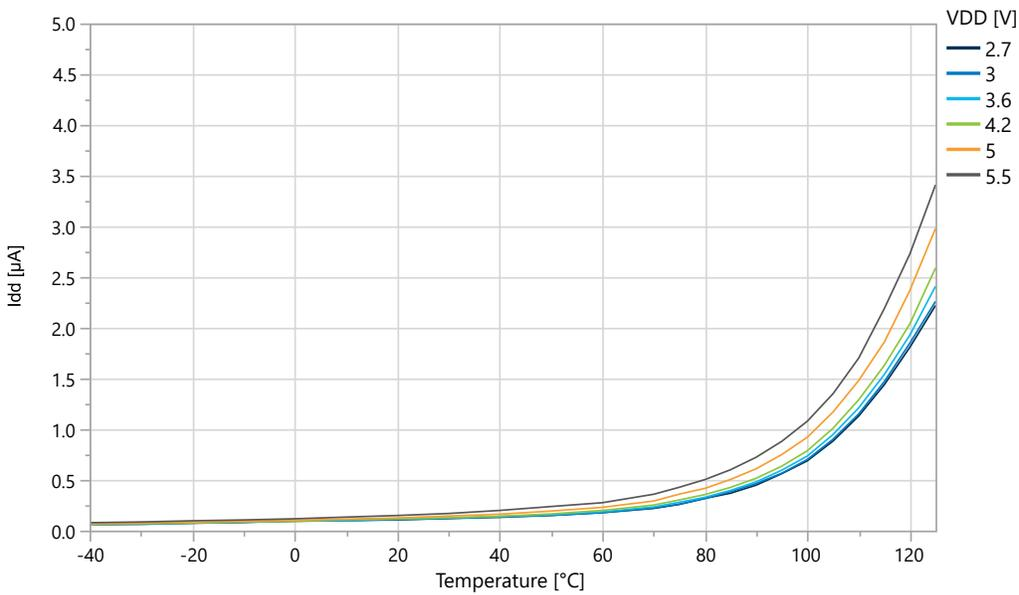
**Figure 33-11. Power-Down Mode Supply Current vs. V<sub>DD</sub> (all functions disabled)**
