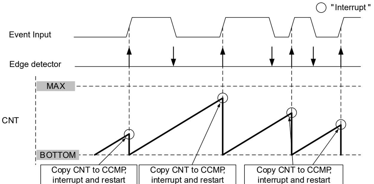
**22.3.3.1.5 Input Capture Pulse-Width Measurement Mode**
