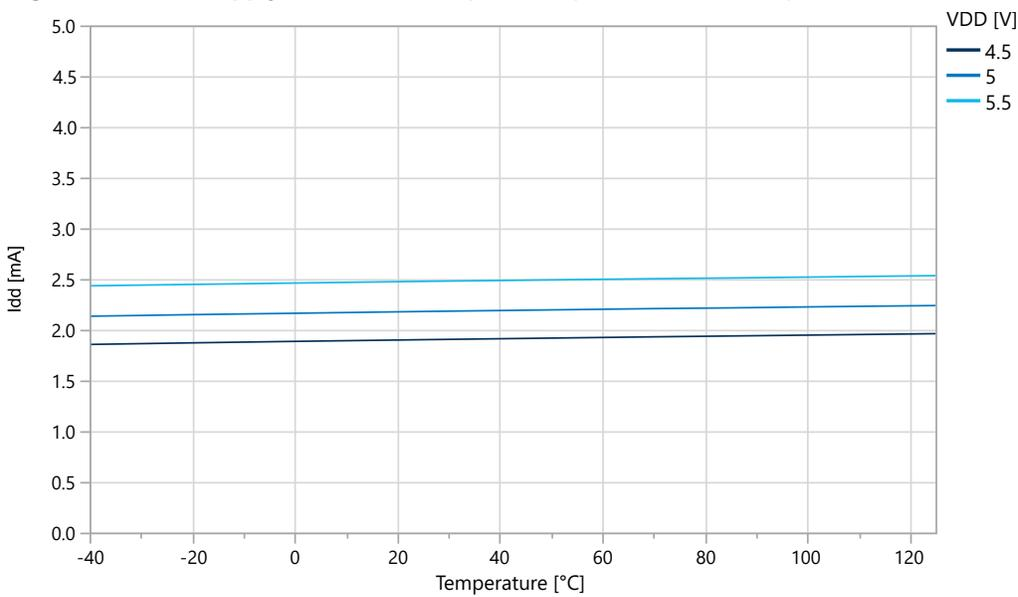
**Figure 33-9. Idle Supply Current vs. V<sub>DD</sub> (f=32 KHz OSCULP32K)**
