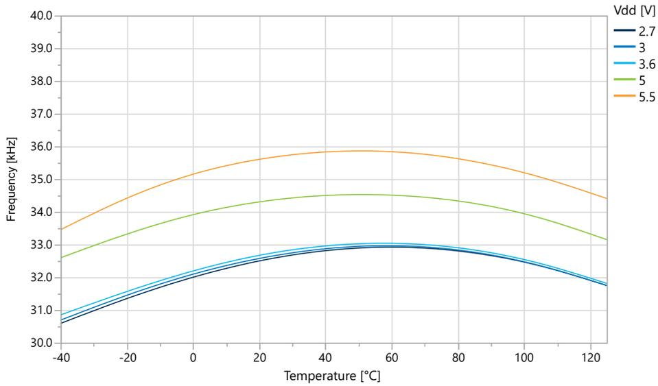
**Figure 33-57. OSCULP32K Internal Oscillator Frequency vs. V<sub>DD</sub>**
