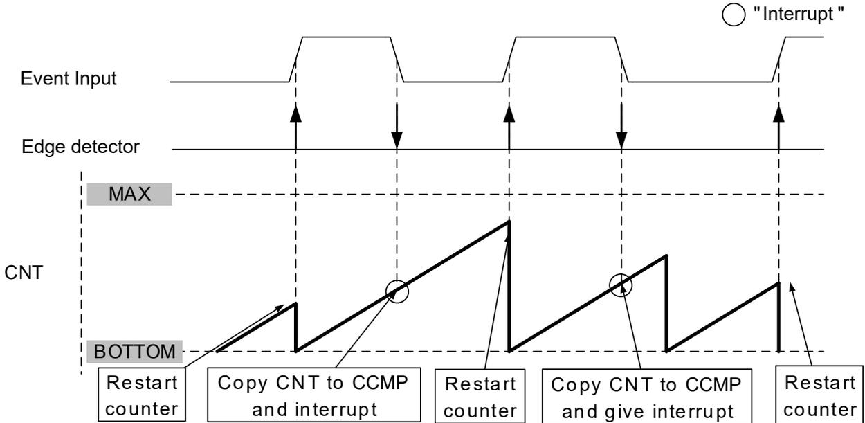
**22.3.3.1.6 Input Capture Frequency and Pulse-Width Measurement Mode**
