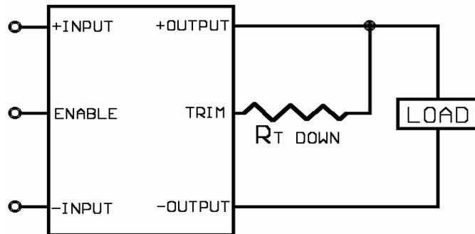
**Figure 5. Trim Connections To Decrease Output Voltages Using Fixed Resistors**
