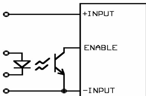
**Figure 3. Driving the Enable Control pin**
