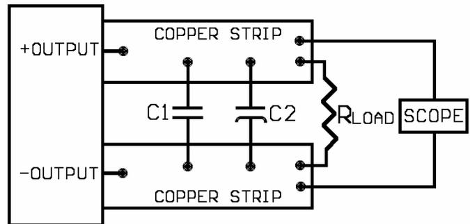
Figure 2. Measuring Output Ripple/Noise
