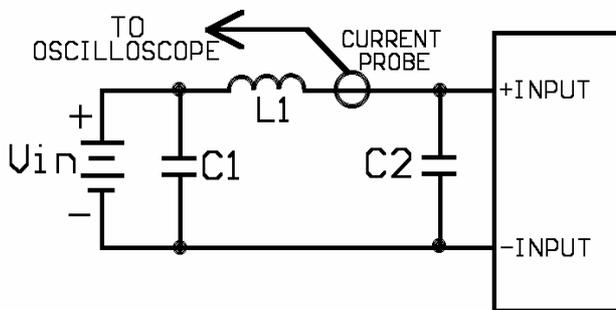
Figure 1. Measuring input Ripple Current
