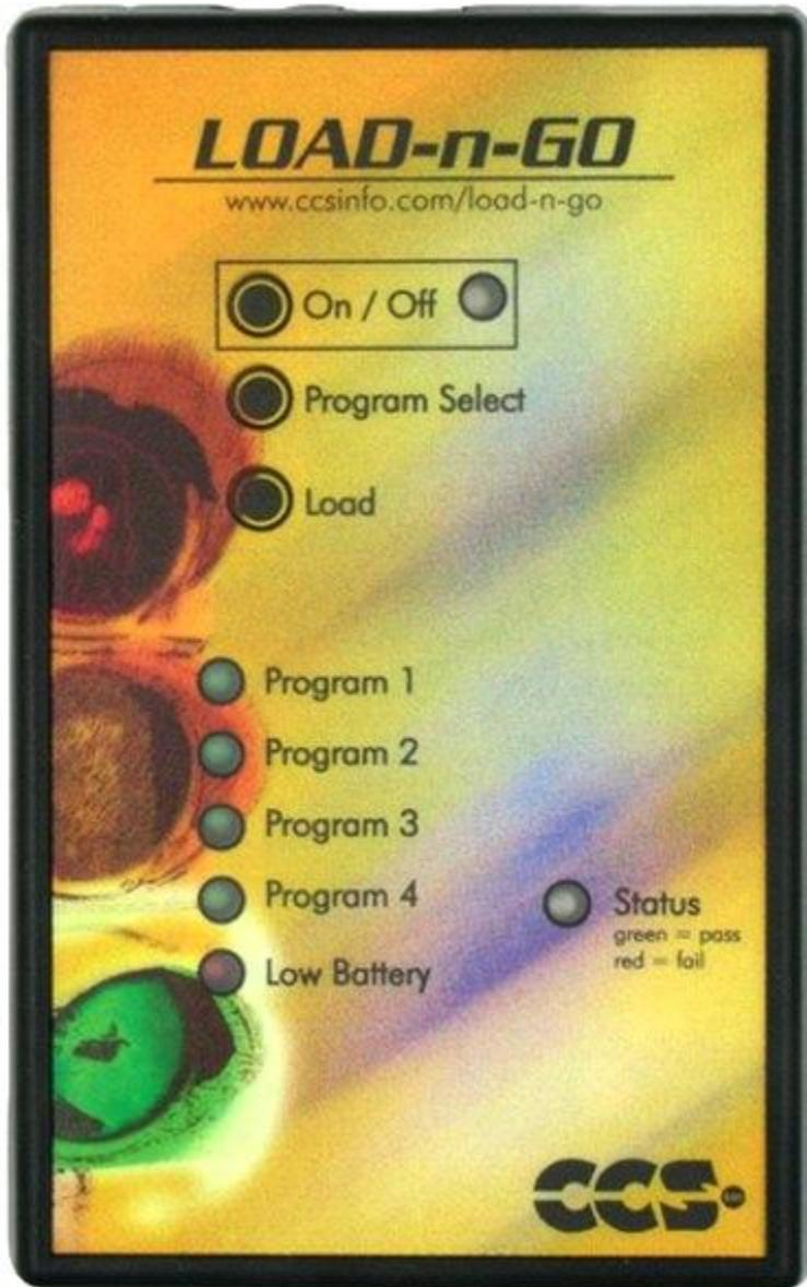
LOAD-n-GO is a hand-held mobile programmer and goes where no PC or laptop has gone before. This device allows for quick field programming of targets with up to four firmware images. The programming process is as easy as 1-2-3 with the LOAD-n-GO. Simply load the program into the LOAD-n-GO via a USB cable, connect to the target and program! LOAD-n-GO debug support covers all targets that have debug mode when used in conjunction with the C-Aware IDE Compilers.
