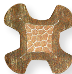
Indenter Crimp Cross-Section Across Axis Figure 2
