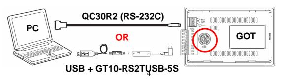
Note that using the GT10-RS2TUSB-5S will require a virtual USB COM port driver to be installed on the PC. The COM port number can be automatically or manually assigned so that it does not overlap with the existing COM port numbers assigned on that PC. When using a Q-Series programming cable, the COM port number already assigned to the RS-232C interface of the PC will have to be checked.
