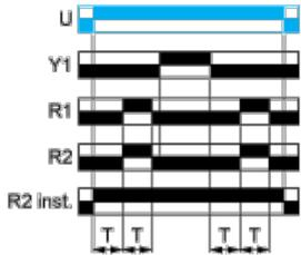
**Function Di: Symmetrical Flashing Relay (Starting Pulse On)**
