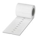
Label, Roll, transparent, unlabeled, can be labeled with: THERMOMARK E.300 (D)/600 (D), THERMOMARK ROLL 2.0, THERMOMARK ROLL, THERMOMARK ROLL X1, THERMOMARK ROLLMASTER 300/600, THERMOMARK X1.2, mounting type: adhesive, Number of individual labels: 2500, text field height: 12.7 mm, text field width: 25.4 mm
