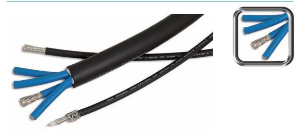
Van Damme now has 2 single flexible digital coaxials to add to the established 4 and 6 way flexible HD Vision low loss multicores. All are suitable for analogue, SDI and HD-SDI transmissions. The 2 single coaxials are based around industry standard RG6/U and RG59/U and their precision construction ensures that electrical performance has not been majorly affected by the use of a stranded centre conductor.
