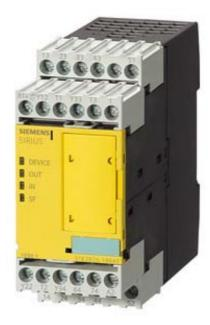
SIRIUS SAFETY RELAY WITH RELAY RELEASE CIRCUITS (RC), UC 24...240V, 45.0MM, SCREW TERMINAL, RC INSTANT.: 2S, RC DELAYED: 2, MK: 3, 8-FUNCTION SWITCH, BASIC DEVICE, MAX. ACHIEVABLE PL TO EN13849-1: E,
