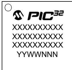
64-Lead TQFP (10x10x1 mm)
