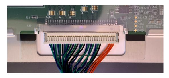
Connect the backlight connector from the driver card to the back of the LCD.
