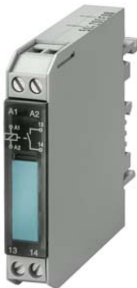
INPUT INTERFACE TERMINAL-TYPE OPTOCOUPLER RELAY 1NO (TRANSISTOR) AC/DC INPUT 24V DC OUTPUT MAX. 30V
