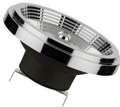
145704 LED Spot ES111 G53 12V DIM 9W (75W) 620lm 927 40° Bridge
