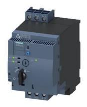
SIRIUS Compact load feeder Reversing starter 690 V 24 V AC/DC 50...60 Hz 0.32...1.25 A IP20 Connection main circuit: Screw terminal Connection control circuit: plug-in, without terminals
