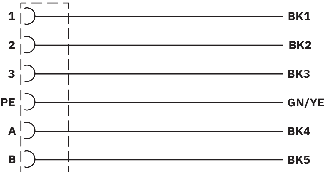
Contact assignment of the M12 socket
