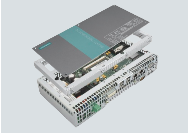
SIMATIC IPC427C with expansion rack; a maximum of 4 PC-IO expansion racks can be stacked.
