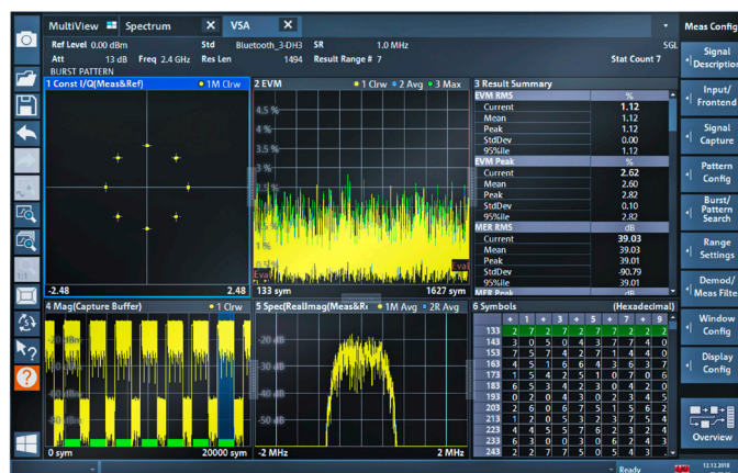
Demodulation of a Bluetooth® signal with the R&S®FPL1-K70 option
