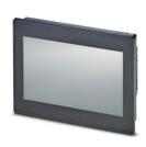
Touch panel with 17.8 cm / 7"-TFT display (analog resistive), 800 x 480 pixel(s) (WVGA), 16.7 million colors, Arm® Cortex®-A7, 528 MHz i.MX6 UL, 2x COM (RS-232/422/485), 1x USB 2.0, Typ A, 1x USB 2.0, Typ B, 1 x Ethernet (10/100 Mbps), RJ45, Windows® Embedded Compact 7 and user software: Visu+. (bus system: without)
