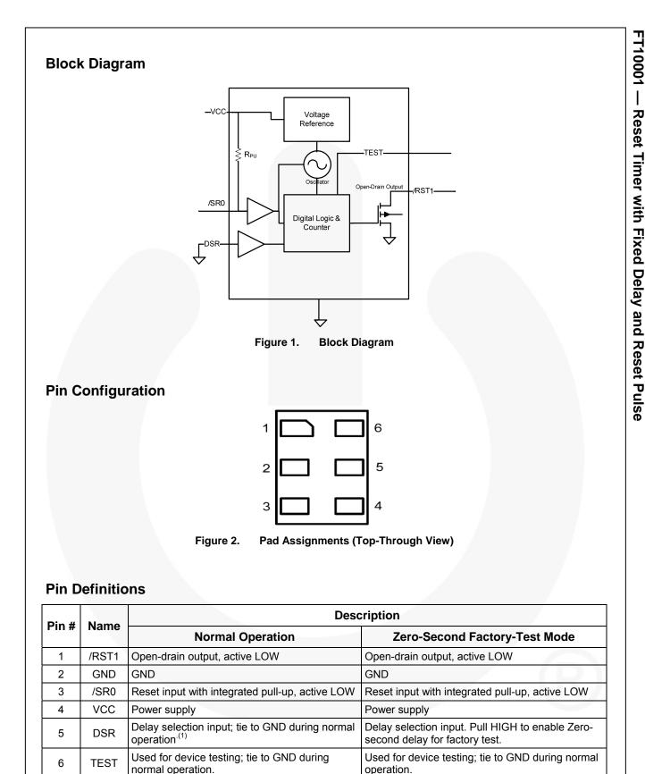
1. This pin must always be tied to either GND or VCC. It must not float.
