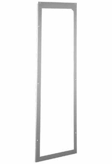
Side Door Adapters are made from 14 gauge steel and finished in RAL 7035 textured light-gray polyester powder paint. They allow the mounting of a standard door to the side of the enclosure. When mounted to the enclosure, they maintain enclosure environmental integrity.
