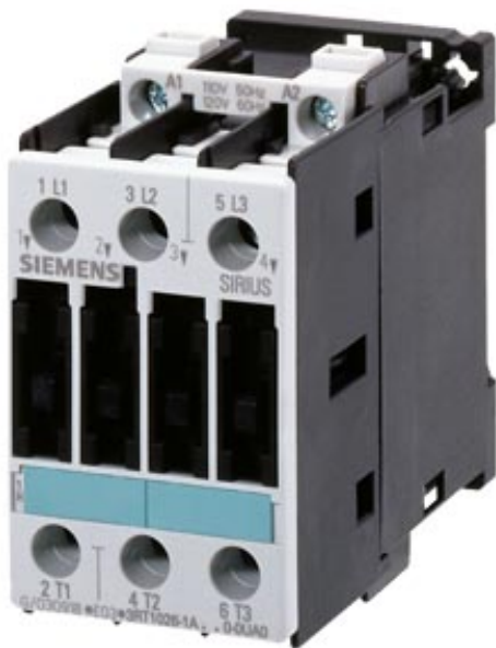
CONTACTOR, AC-3 11 KW / 400 V, AC 400 V, 50 HZ 3-POLE, SIZE S0, SCREW CONNECTION
