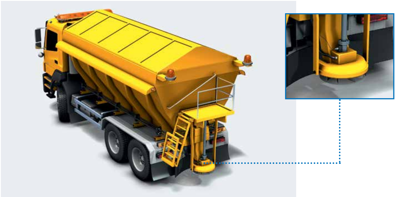
Road Spreader. Proximity sensors control the rotor to ensure the correct speed for spreading of sand and reagents on the roads during wintertime. Extremely tough outdoor application conditions require the highest reliability of the sensors, housing and vibration-resistance of the sensor.
