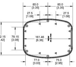
Purchased assembly includes top and bottom cover, 1 removable panel and 6 cover screws (M3-0.5 x 18mm). M3 Brass inserts are installed for cover screws. Enclosure molded from FR ABS (UL94-V0) plastic.
