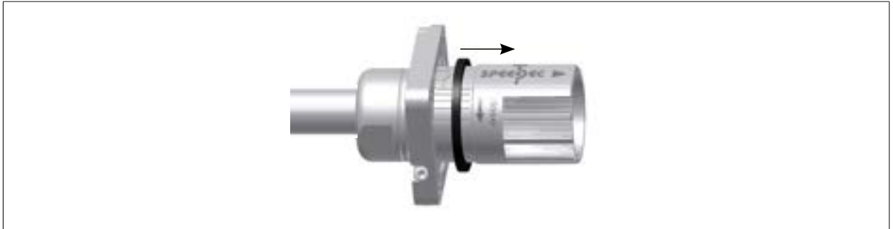
Figure 96: Attaching the metal flange to the connector (rear panel installation)
