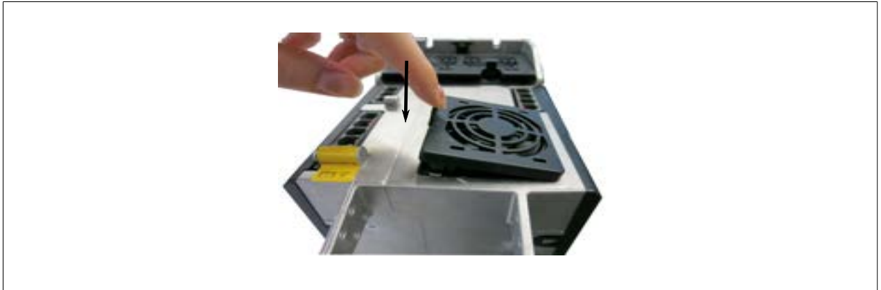
Figure 92: Installing the fan module
