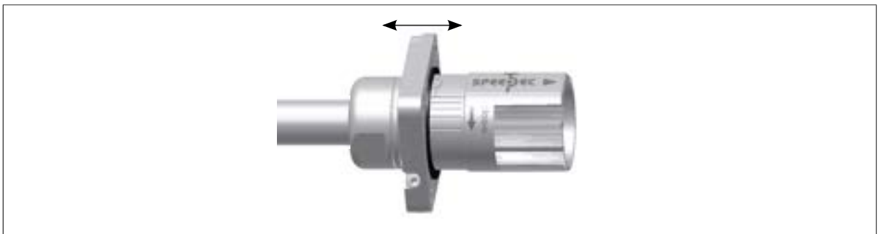
Figure 97: Attaching the metal flange to the connector (rear panel installation)
