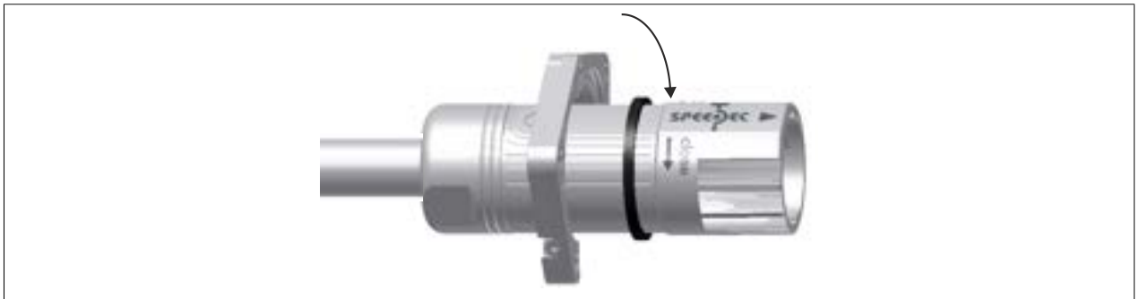
Figure 100: Attaching the metal flange to the connector (rear panel installation)
