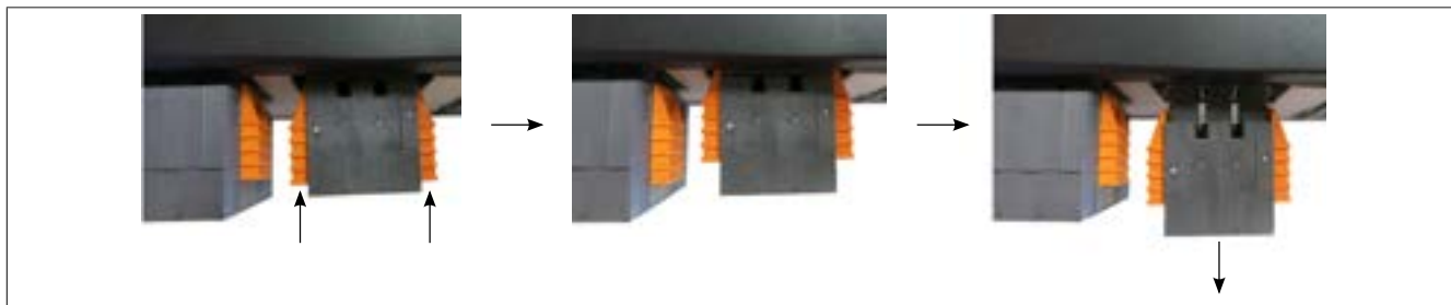
Figure 146: Unlocking and removing 8TB push-in terminal blocks
