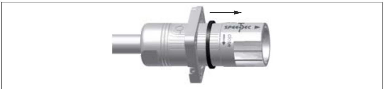
Figure 101: Attaching the metal flange to the connector (rear panel installation)
