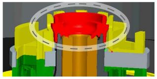
This design concept can solve the moving problem of the motor's components, provide better dust-resistance.
