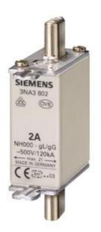
LV HRC FUSE LINK GL/GG WITH NON-INSULATED GRIP LUGS WITH FRONT INDICATOR SIZE 000, 2A, AC 500V/DC 250V
