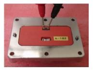
**3.** If voltage across battery pins is either less than 1.8V, or loses power rapidly, or will not charge above 2.5V please contact your distributor for further advice.
