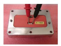
**2.** Check across battery pins with Multimeter set to DC Volts, if battery reads 1.80 to 2.50v place battery in charging station and charge for up to 1 hour, re-check voltage, if reading is now between 2.6 to 3V check battery on unit for power output.
