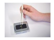
**Note:** For safe transportation, spare fuses are supplied in protective packaging. Carefully remove the fuse from the packaging fuse holder before inserting into the battery.
