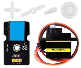
standard cycle of PWM signal is 20ms (50Hz). Theoretically, the width is distributed between 1ms-2ms, but in fact, it's between 0.5ms-2.5ms. The width corresponds the rotation angle from 0° to 180°. But note that for different brand motors, the same signal may have different rotation angles.
